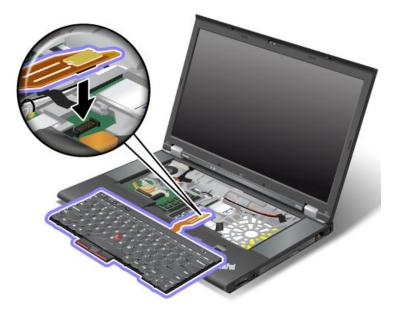
2. Insert the new keyboard. Make sure that the rear edges of the keyboard are under the frame.
